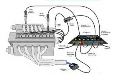
The ignition trigger can be Inductive as displayed above, back probed to the signal side of a coil or with an eCOP (Coil on Plug Adapter).
