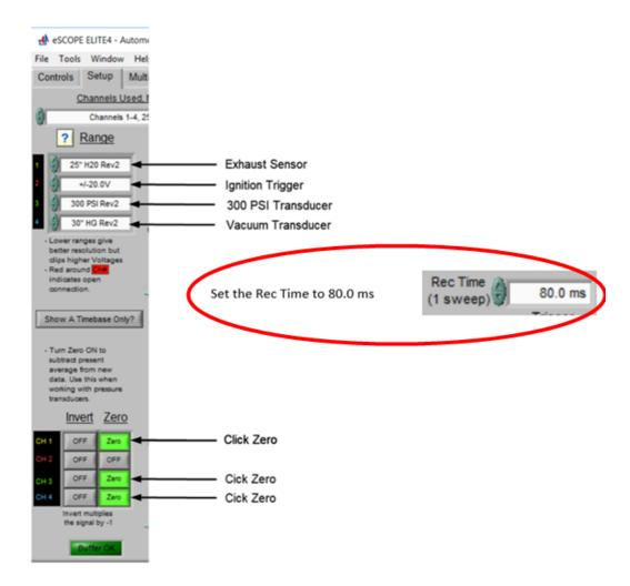
The following two steps are needed to properly capture and diagnose a compression wave form
