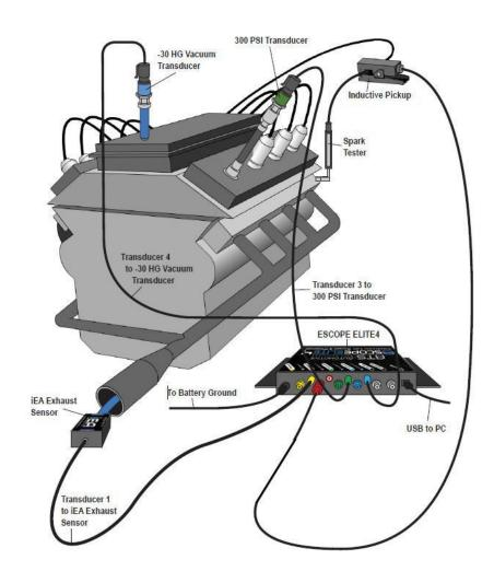
Assuming you are capturing with the eSCOPE and NOT the iEA, set the Range values as displayed below and Zero the transducers in Channel 1,3 and 4. Remember to set the record time to 80.0 ms.
